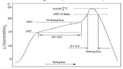
Remark: The peak temperature of soldering heat is 260 +5/-0° for 10 seconds.
